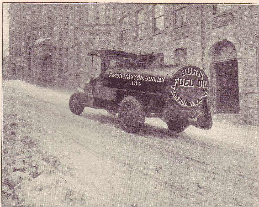
Fuel Oil delivery truck on grade at College Hill, Providence, R. I. Capacity 1200 gallons fuel oil equal to 8 tons of coal.
